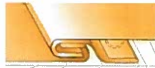
02_FS_04 INTERLOCKING OF SHEETS
