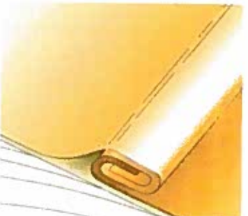
01_BC_30 METHOD 2 DOUBLE LOCK-4
