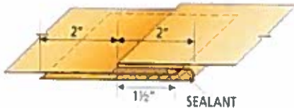
01_BC_21 SLIP EXPANSION SEAM
